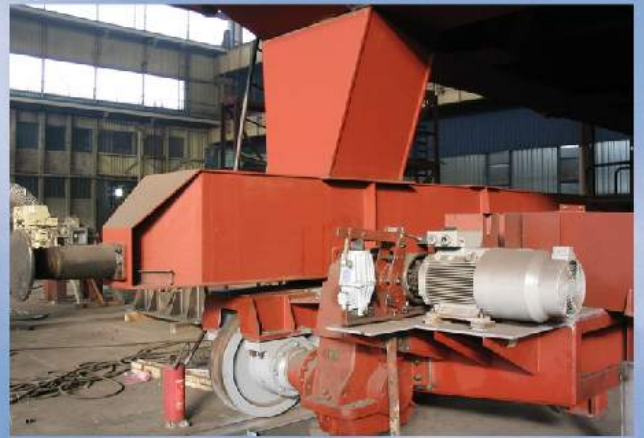
Installation of the electrohydraulic thruster in the draving station on surface mine Gracanica Gacko, Bosnia and Herzegovina- REPUBLIKA SRPSKA
