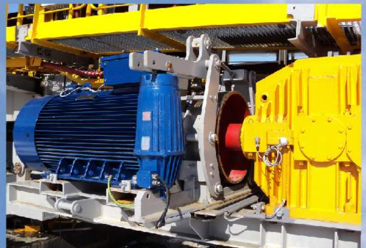
Installation of the electrohydraulic thruster in the draving station on surface mine Gracanica Gacko, Bosnia and Herzegovina- REPUBLIKA SRPSKA
